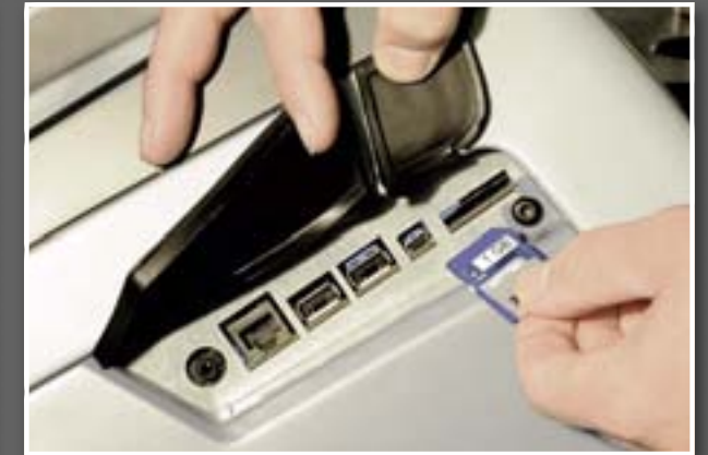
Connectivity: USB ports, LAN network connection, SD card slot for expanding memory
